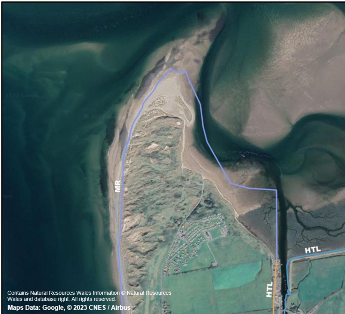
Figure E2 Example of SMP2 Policy Unit data layer, showing how Policy Unit lines are poorly aligned with anthropogenic structures and natural frontages.
