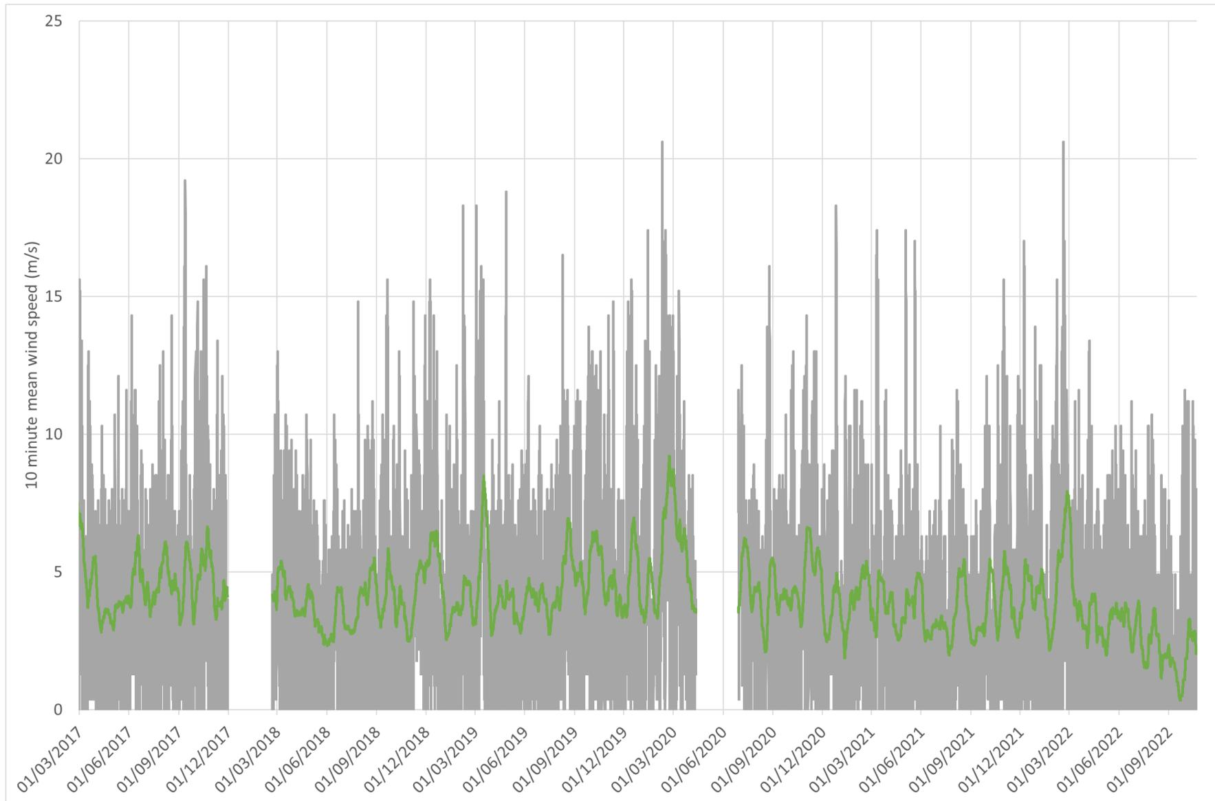
Figure 28: A timeseries of 10 minute mean wind speed from Merthy Mawr, displayed as the raw data (grey line) and the 14 day rolling average (green line).
