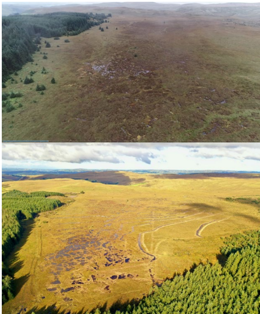
Figure 2. Before (top) and after (bottom) hydrological restoration works at Figyn Blaen Brefi SSSI on the Welsh Government Woodland Estate (WGWE). Photo shows how construction of peat dams and contour bunds reduces water loss and increases bog pool habitat. Photos: Cartwright Associates/Owen Environmental
