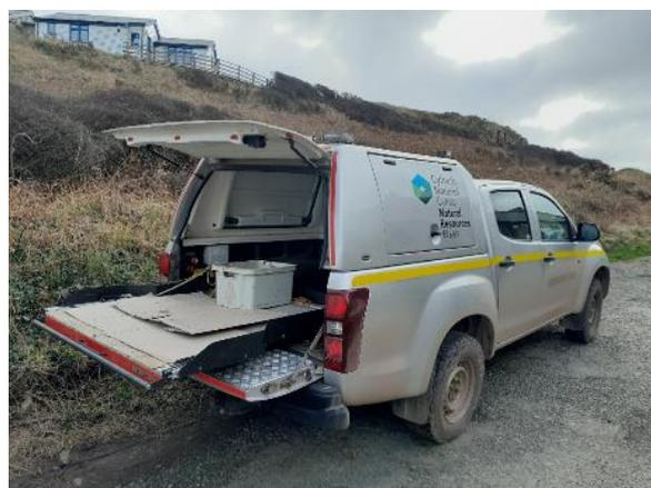
The 'new' fuel bowser with its powered pump has made fuelling Skalmey at Martins Haven much easier and was a particular asset when fuelling at Llansteffan during the SAC infauna survey. The tank is double-skinned to prevent spillages and we carry absorbent materials if the worst should happen.
