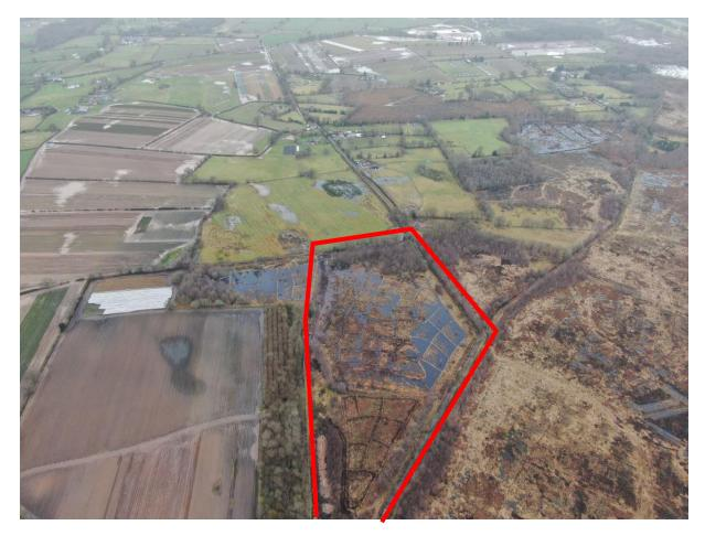
**Figure 7.** Low contour bunding cells installed with NPAP funding in compartment 33 of the Fenn's, Whixall, Bettisfield, Wem & Cadney Mosses SAC during 2020-2021. This site is the third largest lowland raised bog in the UK and work there contributes to the NPAP Lowland Peatlands Priority Action Theme.
