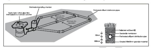
Figure 2: example of a typical drainage field (Building Regulations Section H2)
