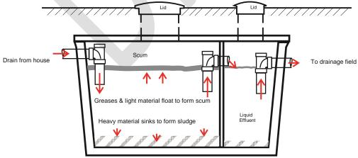
The primary purpose of the tank is to separate solids from the liquid. Solid material settles to the bottom of the tank to form sludge, whilst a scum is formed at the surface. The sludge and scum should be removed periodically and taken away for disposal by a registered waste carrier. The liquid effluent requires further treatment
