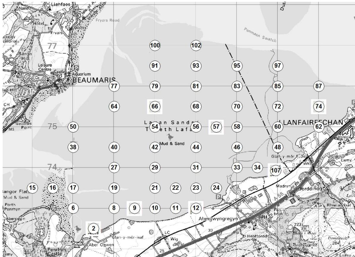
Figure 5 Location of sediment survey stations on Traeth Lafan in 2015. Stations marked with square boxes are those from which core samples were taken for laboratory analysis.
