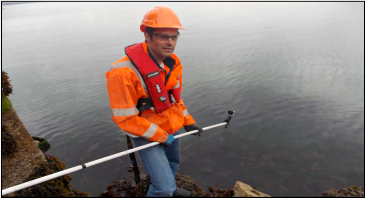
Image 2. Pole mounted Go Pro camera used for shallow subtidal survey
