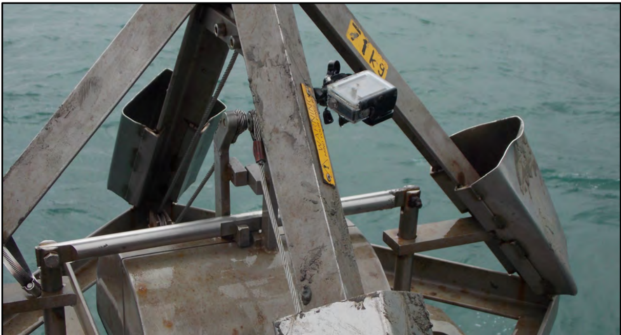
Image 3. Go Pro camera mounted on a 0.1 m 2 Day Grab.
