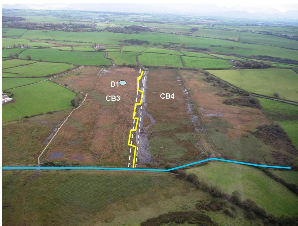
Figure 1. Oblique aerial photograph of Cors Bodeilio taken in October 2011 and looking SE down the long-axis of compartments 3 and 4. The newly opened ditch line (yellow line – diagrammatic only and not exact form) replaces two earlier largely infilled features (dashed white lines) and drains NW into the main axial ditch (blue line) which flows from R to L in this image. Hydrological and rainfall data for location D1 are presented in Figure 2 and Table 3.
