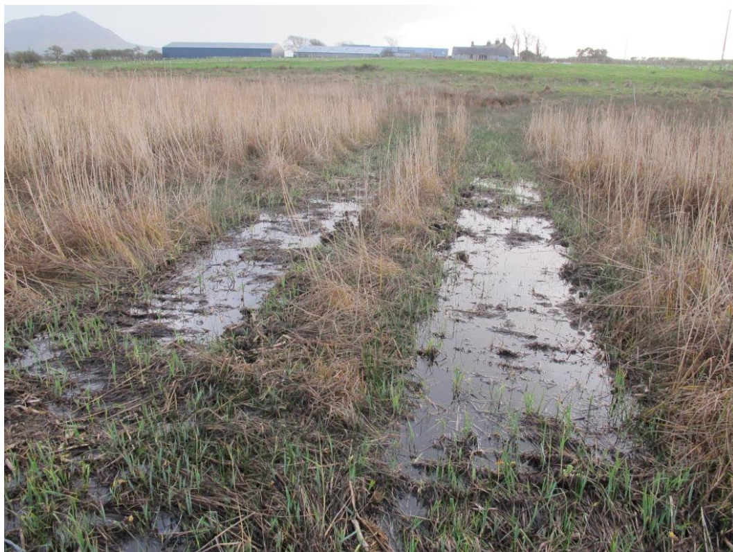
Figure A.3.6. Tracks of 'bog-master' machine on very soft peat. Photo taken from S side of axial ditch looking towards Hirdre Uchaf, December 2013. The vegetation has been flattened but the vegetation raft remains unbroken.
